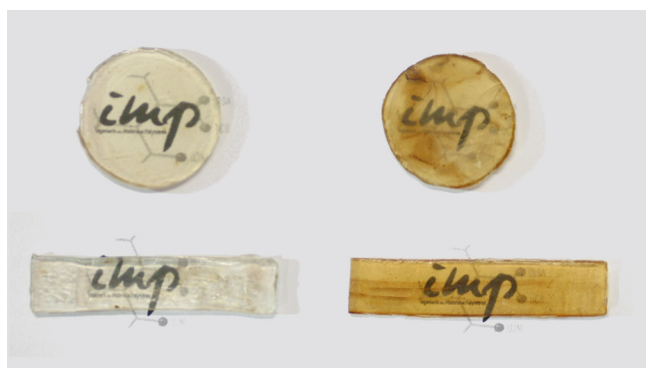
Fig. 3. Visual observations of pressed plasticized samples: (a) CA-DEP-30 and (b) CA-BM-30 processed by melt processing.
